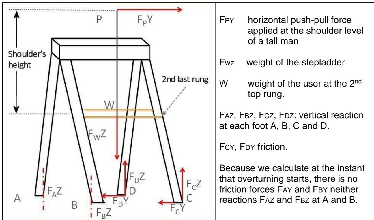
Figure 3. Stepladder with side push-pull
