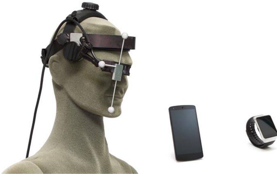
Figure 1. Lite-Eye LE-750 A (Liteye Systems Inc. (2015)) with a custom touch panel. The Lite Eye can also be paired with a smartphone or a smartwatch.
